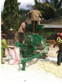
Usually at least six people are involved in operating the machine, two on top and four on the ground. From its design the machine is moved from one area to another manually as shown in picture above. The general dimensions of the machine is 2.2 X 1.8 X 1.2 m. The engine used has the following specifications: Max output power is 24HP@2200rpm, net mass is 194 kg. The total weight of the threshing machine is approximately 650 kg.
