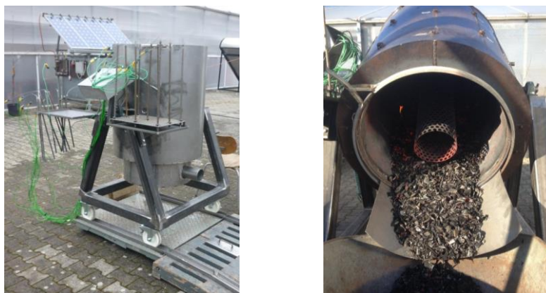
Figure 2.3: Test rig in different positions, left: prepared for filling, probes in transport position, right: tilted for taking out of produced char.
