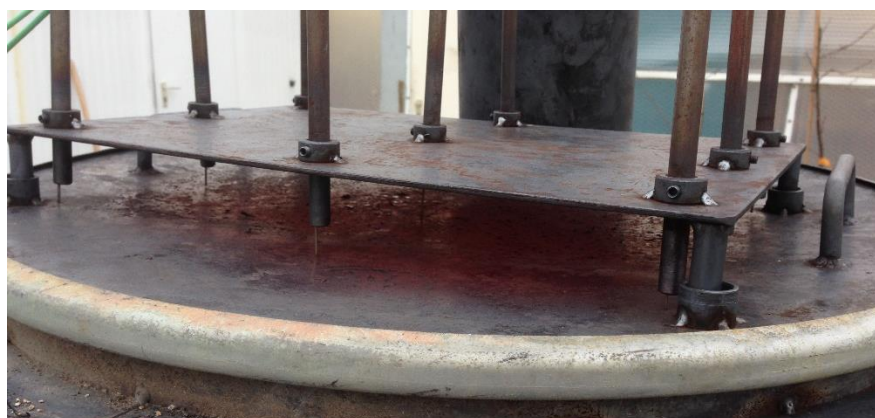
Figure 2.4 Matrix tray with thermocouples and fixing sleeves.
