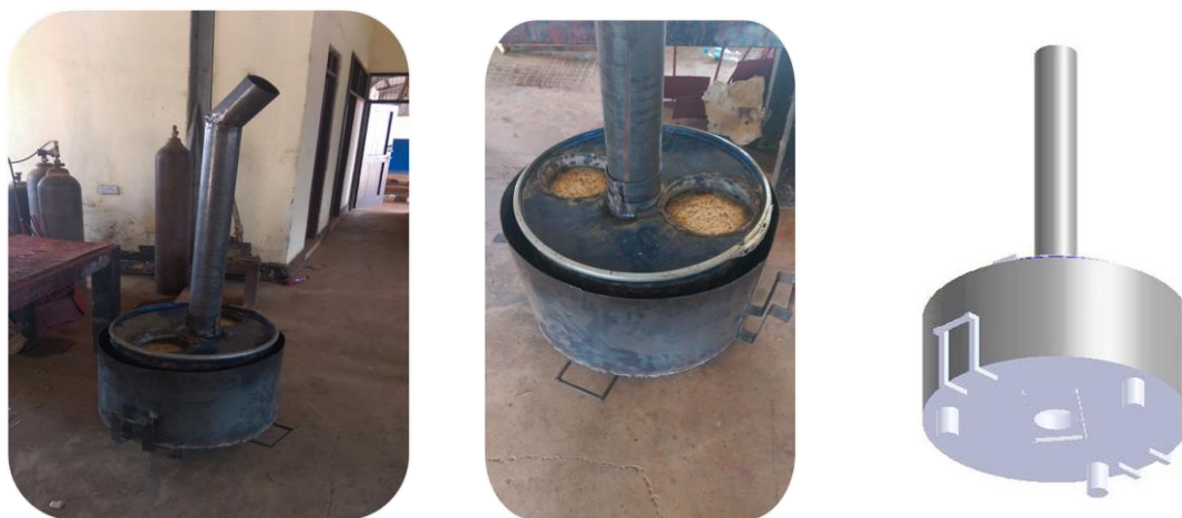
Figure 2.1 Improved TLUD reactor based on the Farmer's recommendation
