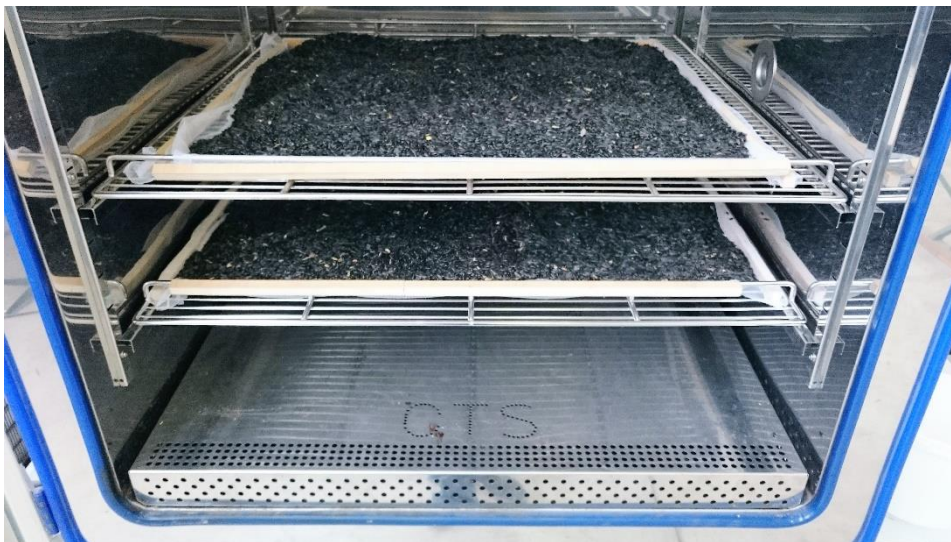
Figure 2.2 Conditioning of HO sunflower seeds in CTS climate chamber
