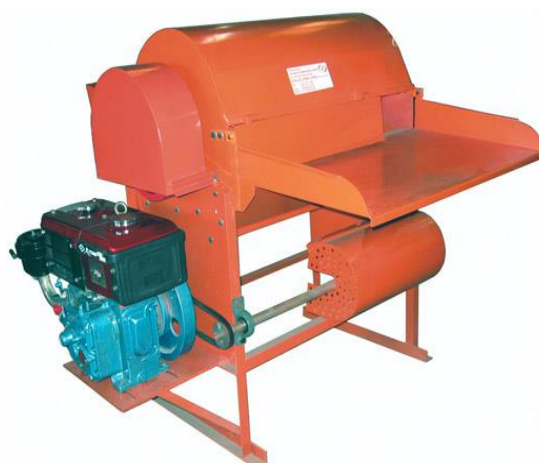
Fig.11. Photographs of an engine-powered sorghum/millet threshing machine made locally
