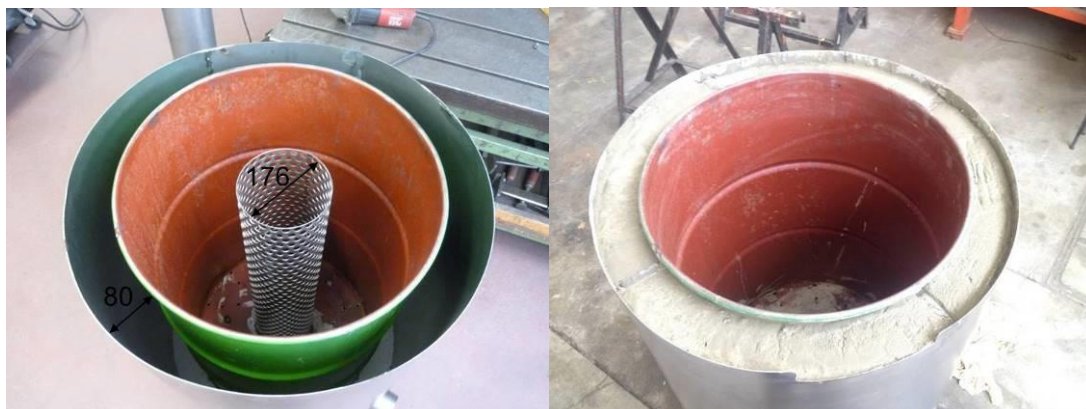
Figure 5. The distance between outer wall of drum and inner wall of ring in mm (left), and insulated TLUD reactor (right)
