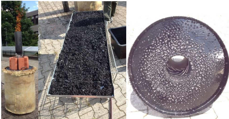
Figure 17. Preliminary test (left), produced char (right), and remaining tar attached on the lid of TLUD reactor at University of Hohenheim
