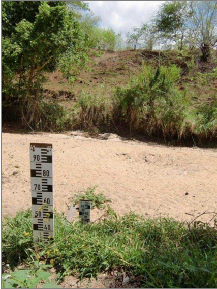
Fig. 6: River water level gauge at the seasonal Ngerengere river, Tanzania
