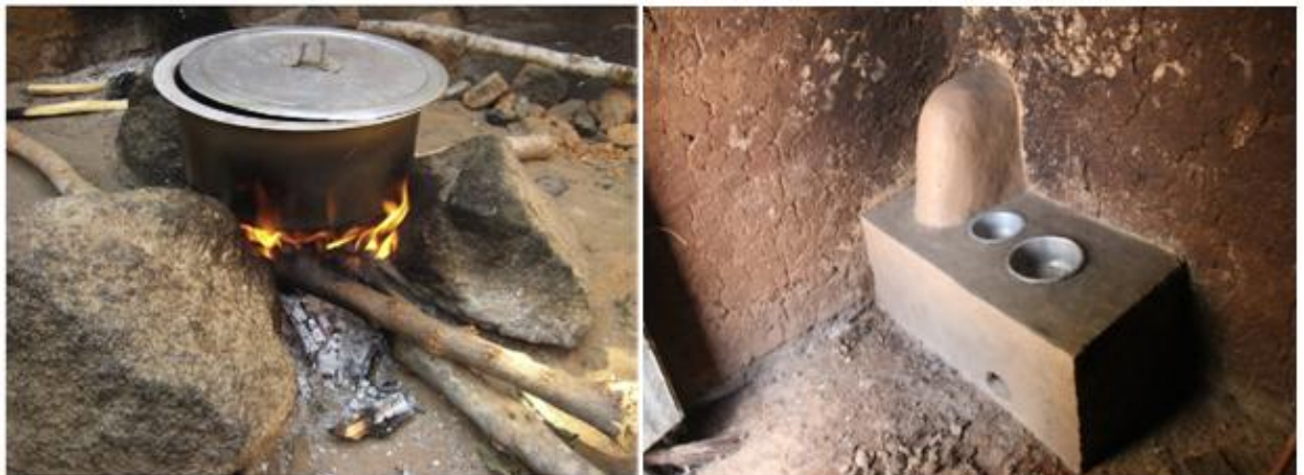
Figure 1: 3 stone fire stove used traditionally in Tanzania (left) and Improved Cooking Stove constructed in Idifu by Trans-SEC (right).
