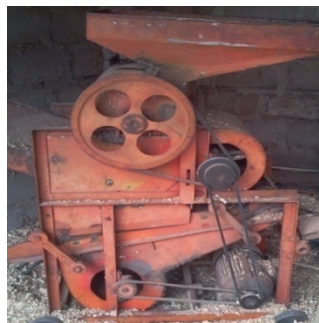
Figure 6: A motorized groundnut sheller at Mbande village, Kongwa (Mutabazi and Rusike, 2012)
