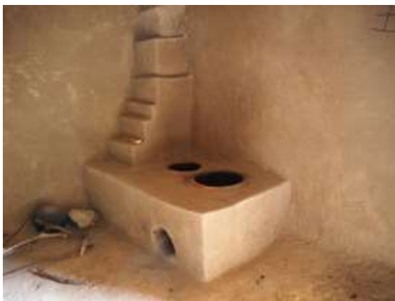
Figure 10: Example for design of new ICS including “changes” of chimney and height of stoves
