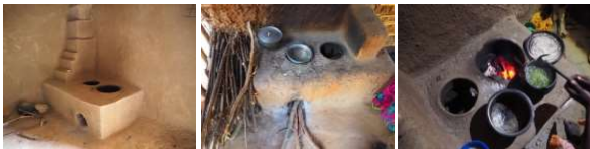
Figure 1: The mud stove of Trans-SEC - a variation of the rocket Lorena stove originally developed from APROVECHO
